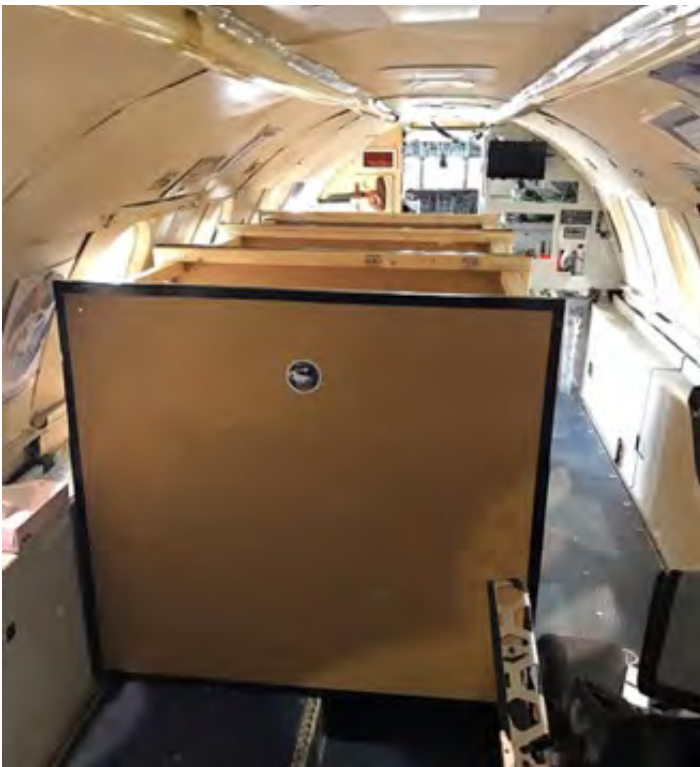
Fig. 1: (left) ASEC chamber mock-up in the cabin of the NRC-CNRC Falcon 20 reduced gravity research aircraft during an October fit check. (right) Preliminary design of the segmented ASEC chamber, enabling installation of a very large chamber volume in a small aircraft.
