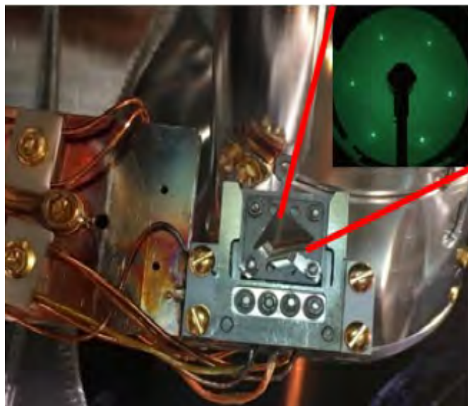
Figure 3: Sample holder and LEED pattern (upper right) of single crystal Ru(0001) thin-film sample for growth of lunar surface surrogates.
