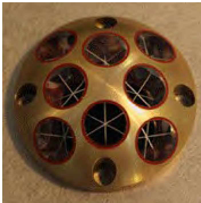
LaRRI (the base of the dome has a diameter of 54 mm; each CCR has a front face diameter of 1/2 inch)
