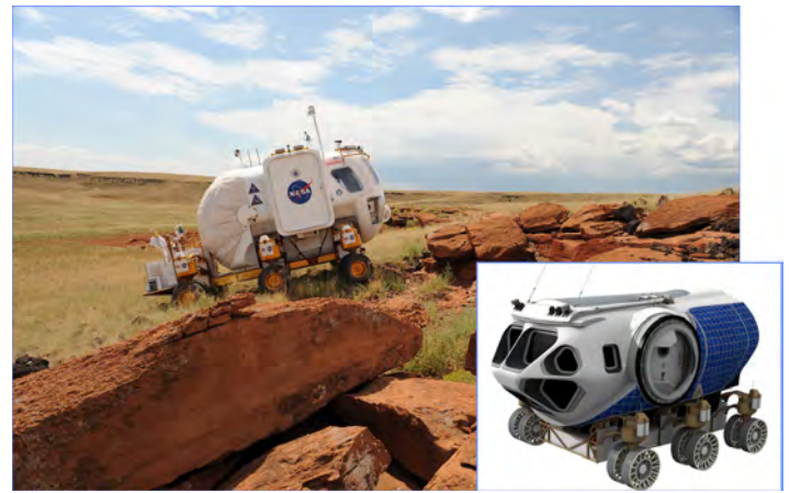
Figure 5. A review of the operational capabilities of the Lunar Electric Rover in field tests, coupled with an analysis of reasonable lunar surface traverses, confirmed that a pressured rover with suitports provides a mobility solution that is easier on crew and enhances their productivity.
