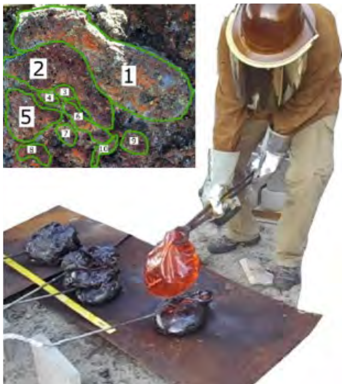
Figure 3. Experimental spatter bombs created at the Syracuse Lava Project are shown being stacked with thermocouples between each clast. The cooled product mimics the appearance of natural spatter clasts (insert) from Idaho.
