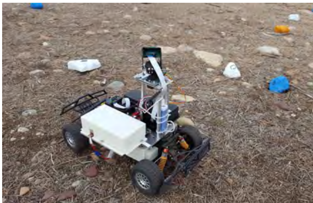
Figure 2: Close up view of the student-built COTS rover at the University of Colorado Boulder. The forward facing stationary camera is mounted at the front and the top camera is mounted on two servos for manipulation. The various electronics controlling the rover are housed underneath the white and black protective shields. The painted rocks are exploration targets for this teleoperated rover.
