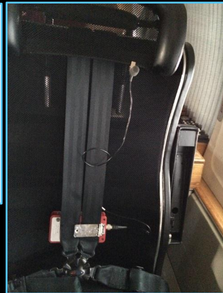
Dosimeter noise recorder, trail aircraft cabin installation
