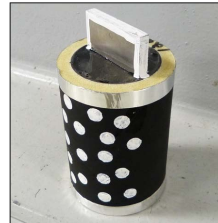
Sharp Projectile – 0.75lbs 2” x 2” x 0.25” Titanium Plate Flexane® 94 – 3” diameter
