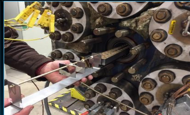
Sample holders using the GEER center port
