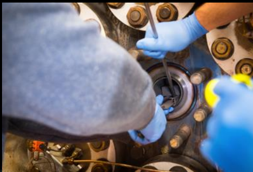
Removing sample holder from vessel
