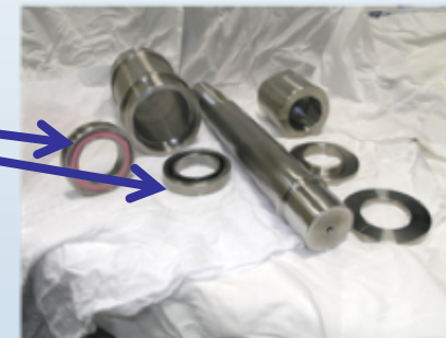
DA Centrifuge Bearing Test Rig Spindle Components
