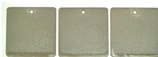
Figure 9. Antimicrobial Hydrophilic Coating on Test Panels
