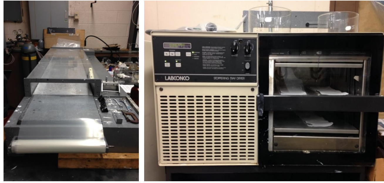
Figure 6: Freeze casting table displaying mylar carrier and granite casting surface.
