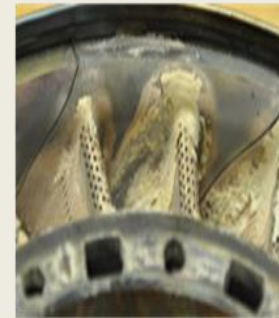
Typical build-up on vane
