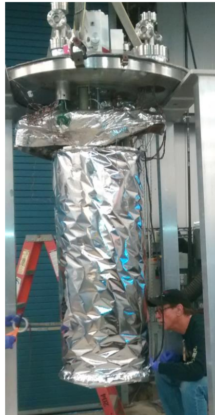
Figure 3: Technicians installing a SHIIVER test coupon blanket onto the calorimeter.
