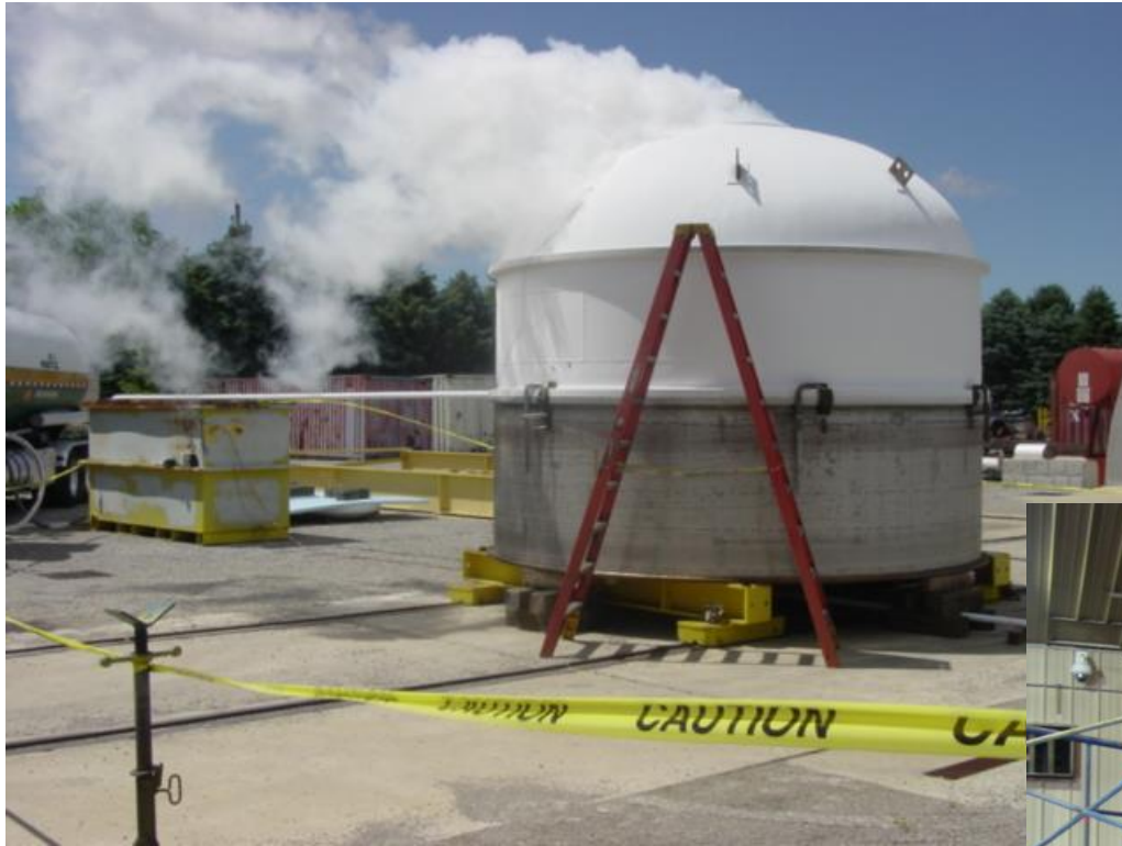
SHIIVER Tank During Cold Shock
