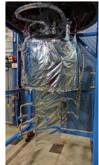
Subscale vapor cooling test (skirt section hanging below calorimeter)
