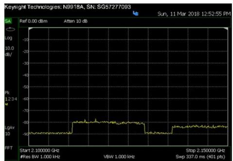
LTE/WiFi spectrum covering 2.1 GHz to 2.15 GHz recorded in the lab by a spectrum analyzer. The resolution BW is 1 kHz, and the overall BW is 50 MHz.
