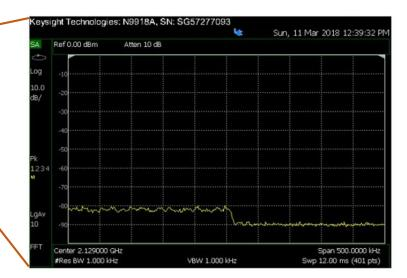
Zoom in on the spectrum analyzer plot to obtain a similar bandwidth (500 kHz)
