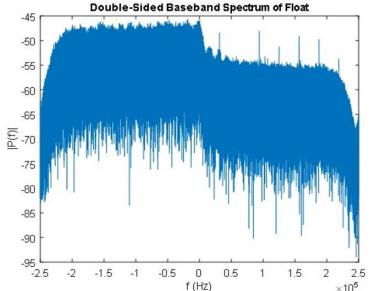
The same spectrum captured by the RF channel sensing payload - measurement time 3 min, 7.2 million complex samples
