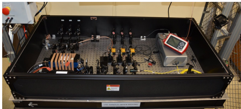
Figure 4. Air-side laser injection setup.
