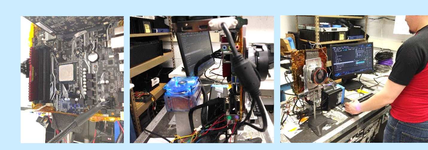
Figure 5: Reverse Side Modifications 180W Cooling on Lidded AMD Ryzen CPU
