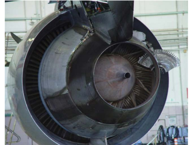
Turbine Disk Failure – June 2, 2006
