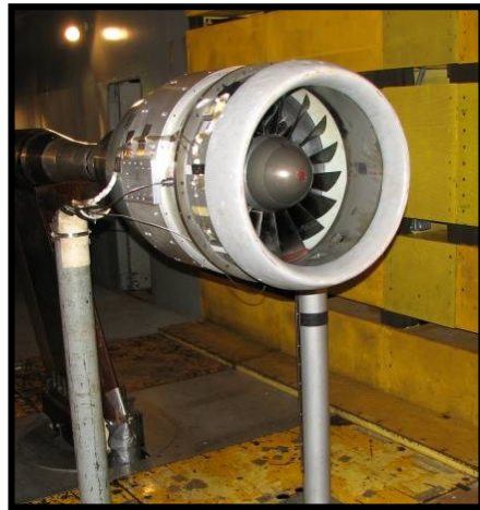
Blade Tip Clearance Evaluation on NASA Turbofan
