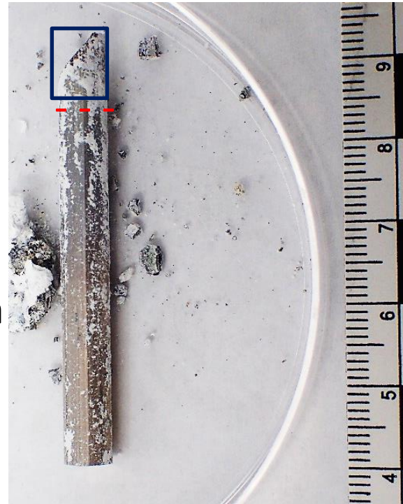
WE43 rod analyzed with CT. Red dotted lines indicates areas of transverse sectioning on CT images.
