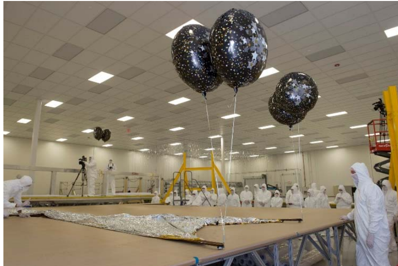
Figure 15. Boom tip gravity offloading.
