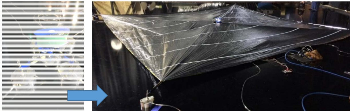
Figure 9. First sail deployment test: half scale 3D-printed prototype.
