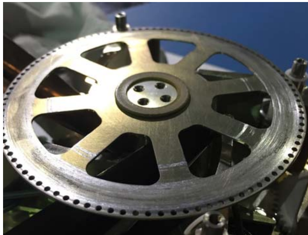
Figure 3. As-built air gaps. Note the near line-to-line contact between the gear and base plates
