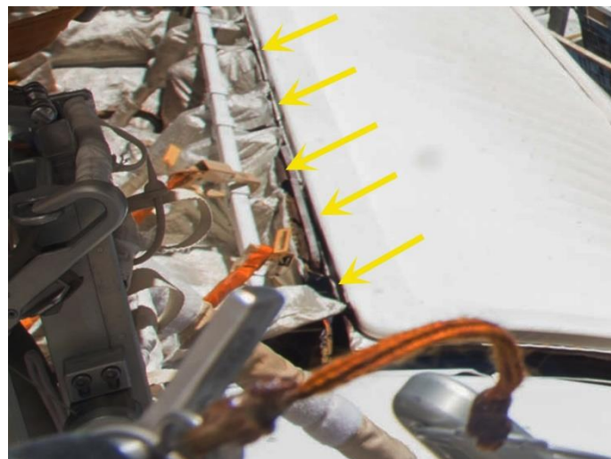
Possible MLI Lifted on FGB; Plane 3 /Zenith
