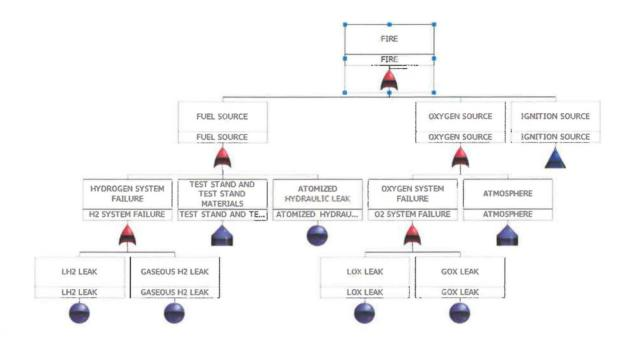
Due to the flat structure of RCAT, the whole FTA cannot be represented in this small space, while the Windchill FTA can fit quite comfortably. This is due to the fact Windchill FTA has transfer gates (represented by a triangle) which link to stand alone trees. The gate content is displayed elsewhere, allowing representation of a complete branch. Windchill may also linked to SSC's DDMS.
