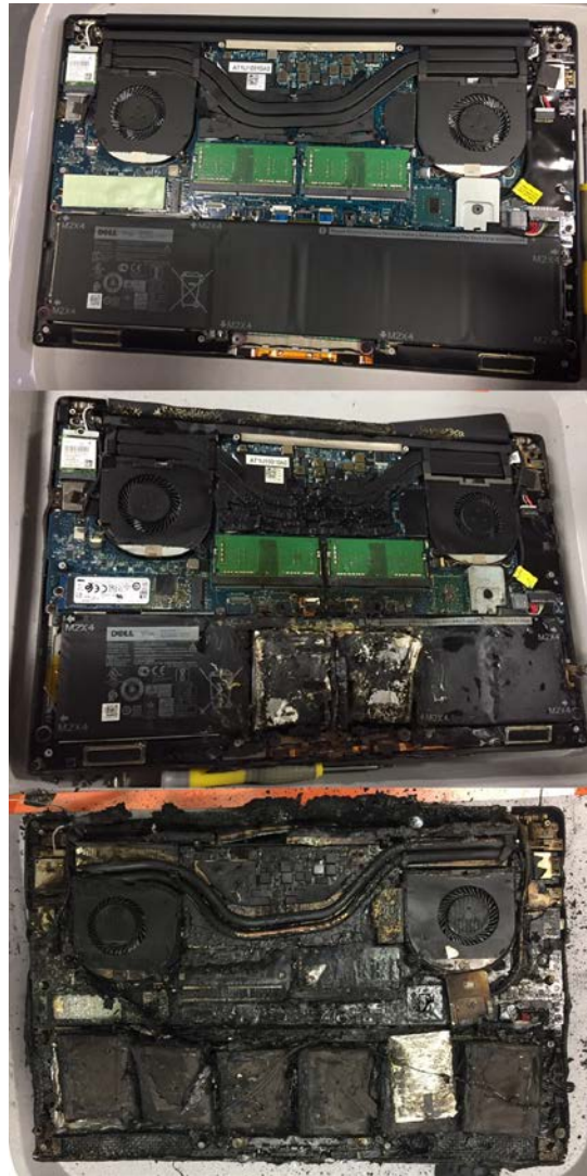
Figure 5. Dell XPS 15 six-cell battery configuration and thermal runaway propagation. Pre-test Li-ion battery pack configuration of six cells configured in-line (top), post-external heating and thermal runaway with Water Spray PFE engagement (center), post external heating and thermal runaway propagation to all battery cells (bottom)
