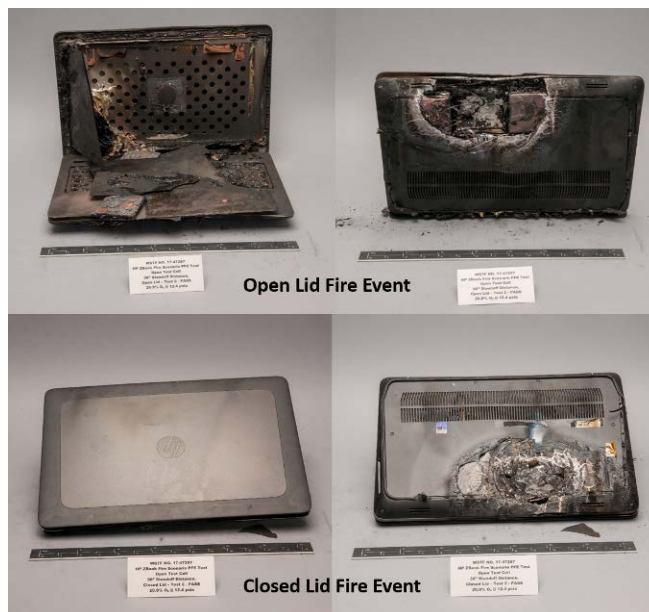
Figure 2. HP ZBook 15 G3 Notebook post stored-energy battery fire and Mg case ignition.
