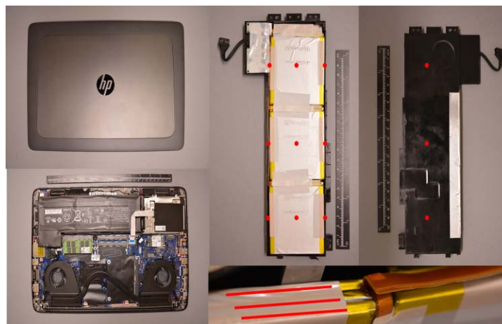
Figure 4. HP Zbook 15 G3 nine-cell battery configuration. Three rows, each row containing three stacked batteries. Red dots indicate thermocouple placement for event monitoring.
