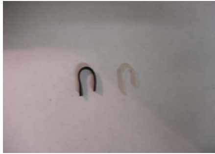
Figure S2. Shape memory effect of LaRC-SMP and LaRC-SMPC.
