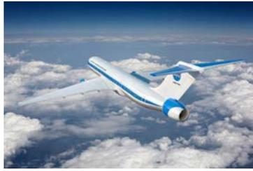
STARC-ABL – Partial Turboelectric
