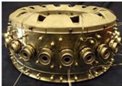
**Fig. 4. NASA/PW/UTRC Axially-Controlled Stoichiometry Low-Emissions Combustor showing multiple fuel ports**
