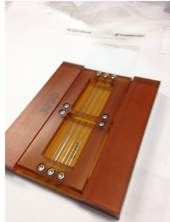
LMM-B1 Sample Assembly Prototype that will contain up to 8 square 100mm capillaries
