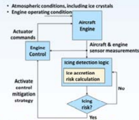
Control-based icing risk detection and mitigation architecture
