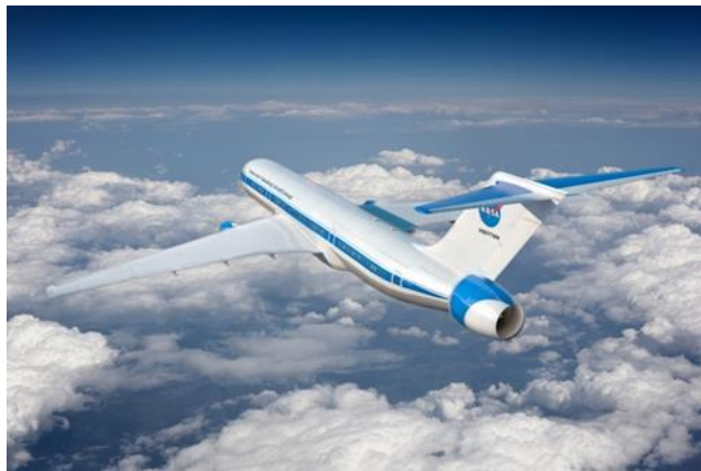
Figure 1: NASA's Starc-ABL concept aircraft with a hybrid electric propulsion system which includes two turbofan-engines and an aft-mounted BLI propulsor [10].
