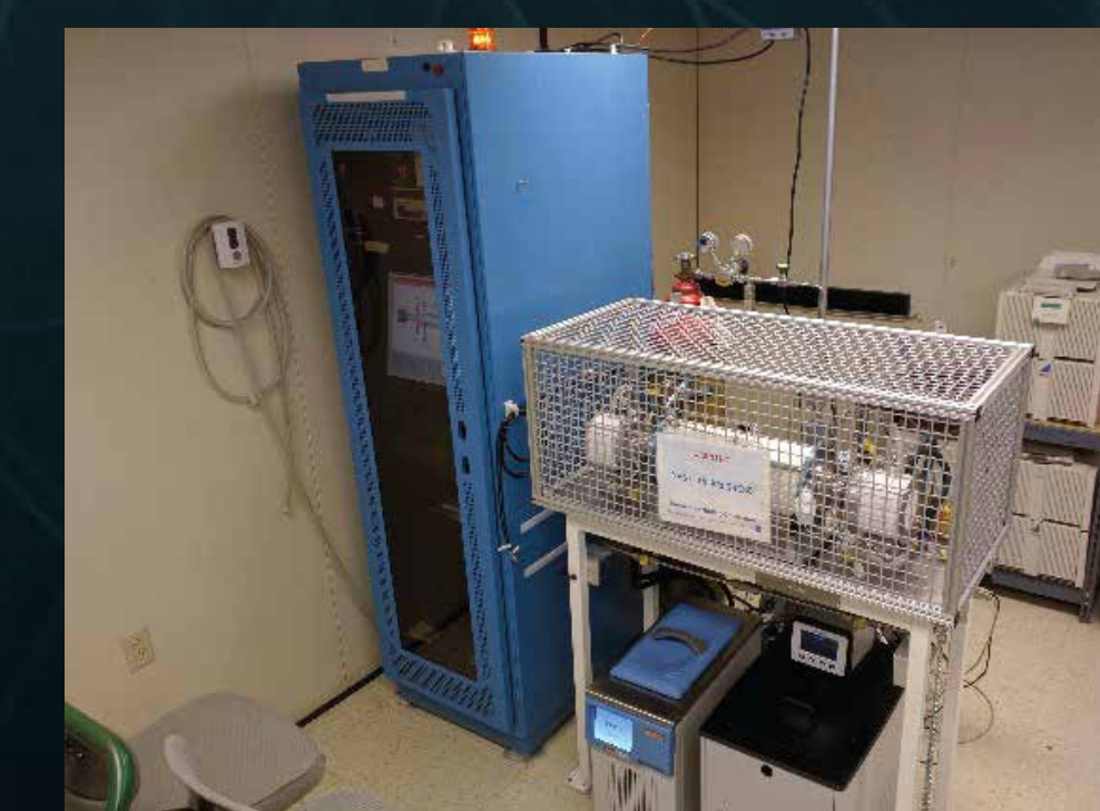
Flexure-bearing Stirling convertor continuous operation test article
