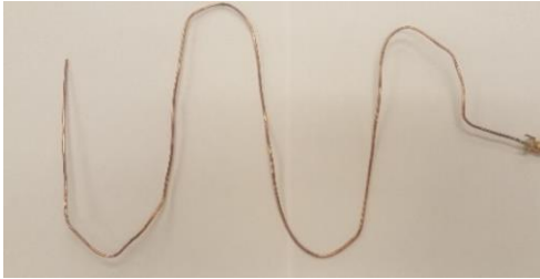
Fig. 4 The 30 cm long, curved wire antenna
