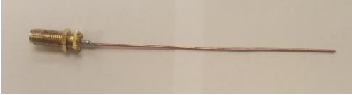
Fig. 3 The 104 mm short wire antenna
