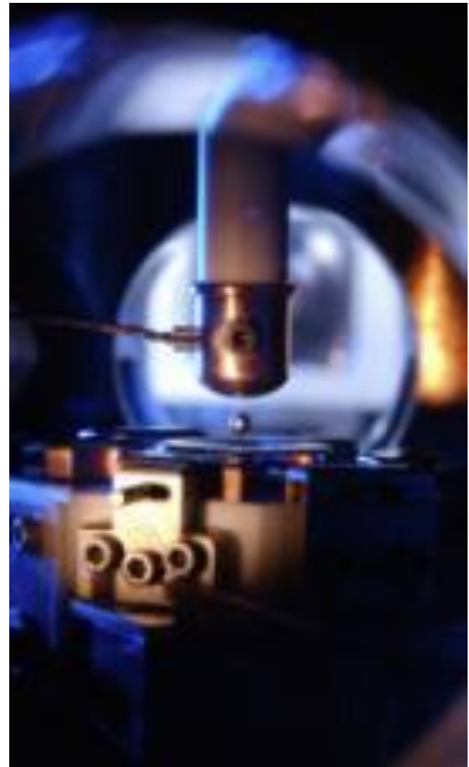
Levitated sample in MSFC ESL
