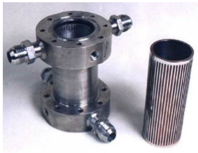
Fig. 12: Combustion chamber liner (with cooling channels) and test assembly
