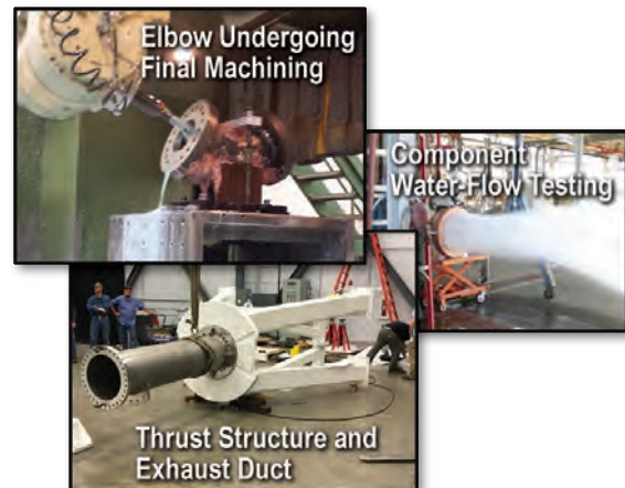
FIGURE 4. ABEDRR hardware fabrication in work.
