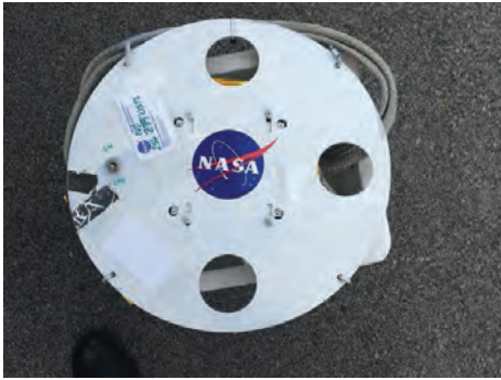
FIGURE 2. Balloon payload with PULSAR underneath plate.
