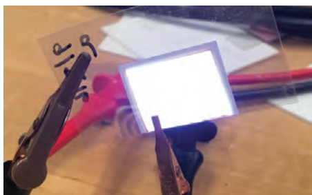
FIGURE 1. Screen-printed EL device made with MSFC dielectric.
