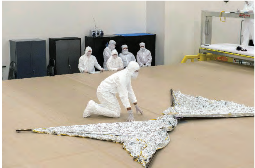
FIGURE 2. The partially unfurled NEA Scout solar sail during a deployment test.
