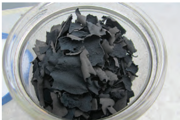
FIGURE 3. A sample of carbon produced in the pH Matter Carbon Formation Reactor. The carbon formed as very fragile flakes with specks of catalyst intersperse within the flakes.
