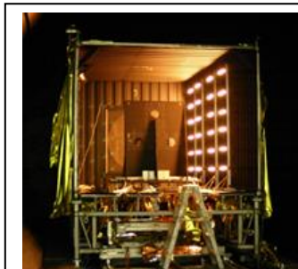
Figure 8: Solar Lamp Array added to MSFC XRCF.
