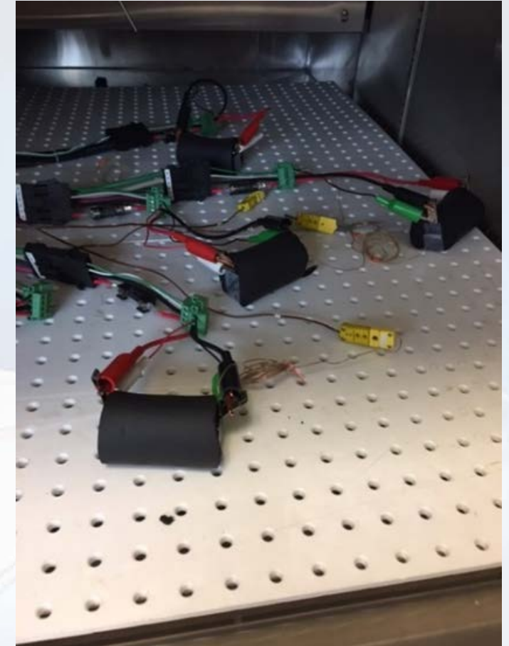
30Q cells tested under flight simulated environment
