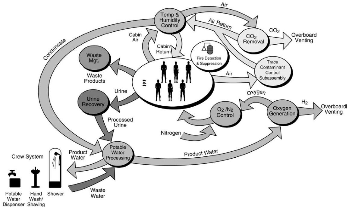
Figure 3. Environmental Control and Life Support System Diagram.<sup>5</sup>
