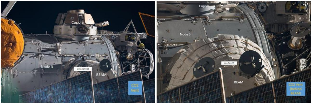
Figure 5. Installation and Expansion of BEAM in relation to Node 3 CO<sub>2</sub> Vent Line.<sup>13</sup>
