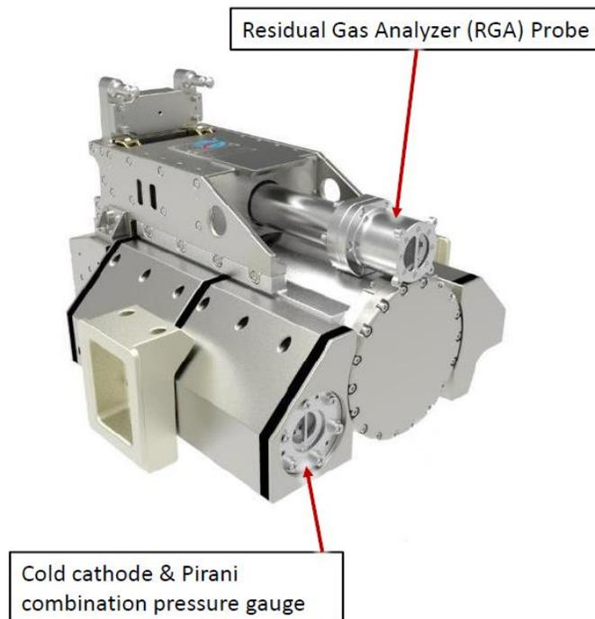
Figure 2. Robotic External Leak Locator.<sup>2</sup>
