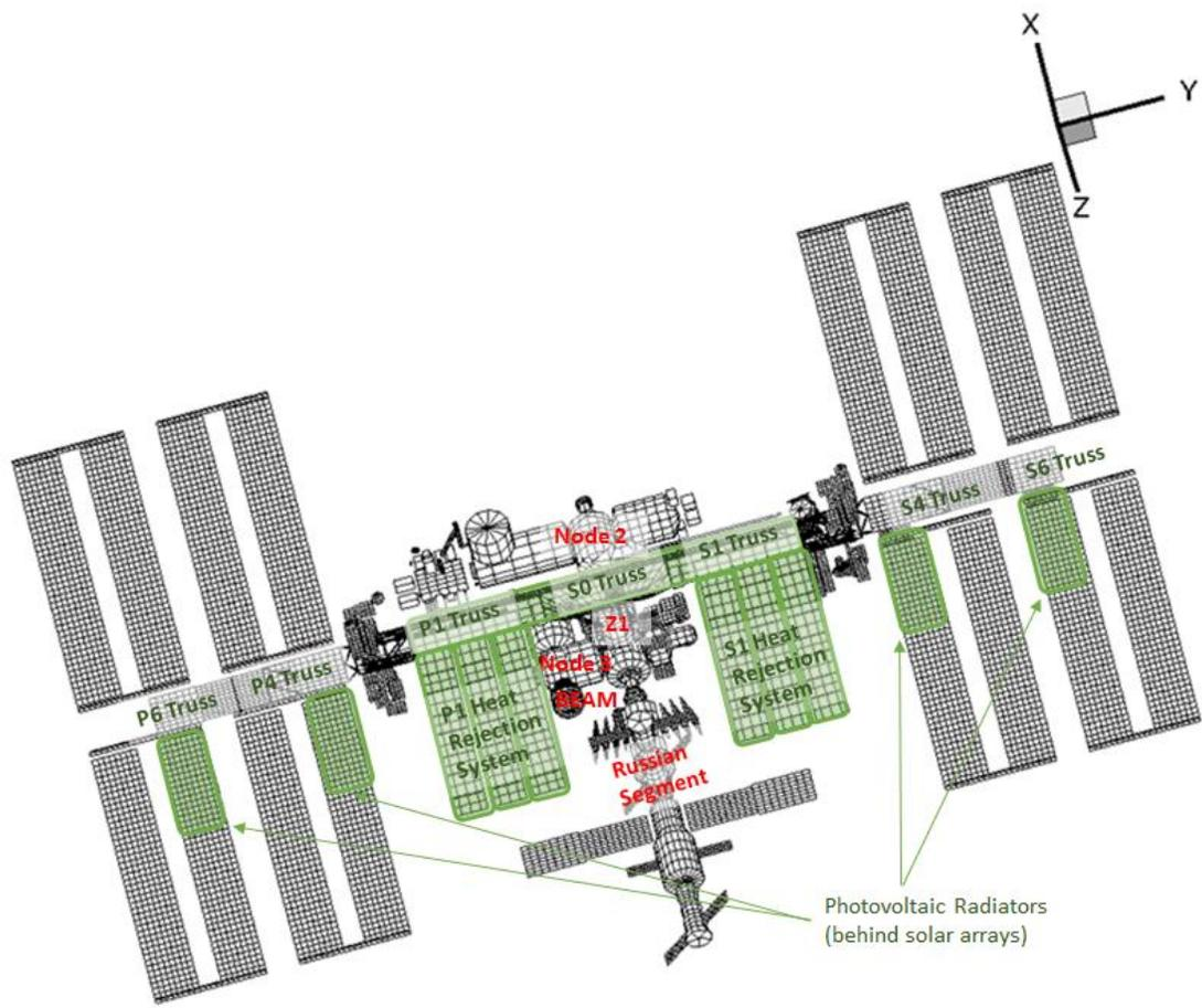
Figure 1. Locations of External Ammonia Coolant Loops (highlighted green) on ISS.
