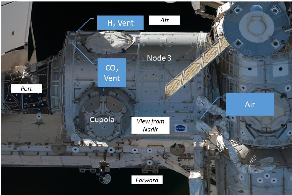
Figure 4. Node 3 Vent Locations prior to Bigelow Expandable Activity Module Installation on ISS.<sup>13</sup>
