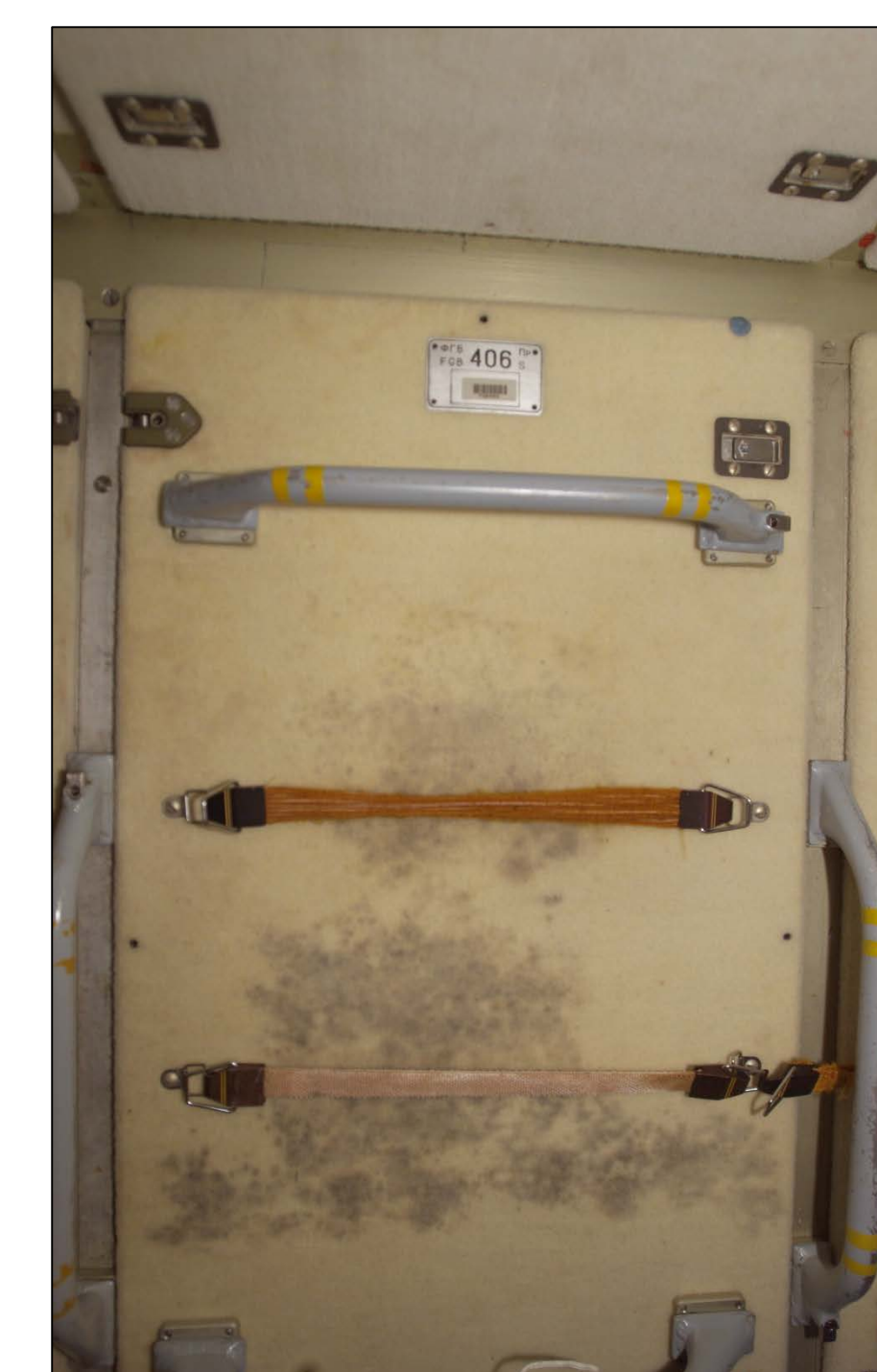
Fungal contamination on a panel in the Russian Functional Cargo Block module (NASA ISS009E28777)
