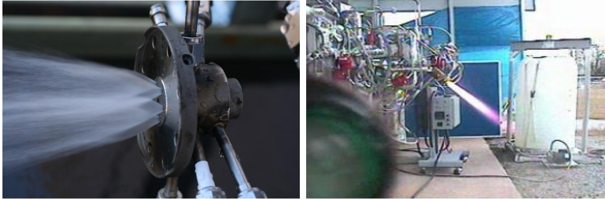
Figure 8. Water Flow Test of Nanolaunch Injector (left); Hot Fire Test (right).
