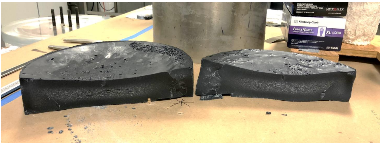
Figure 11 Freezer grain after warmup.
