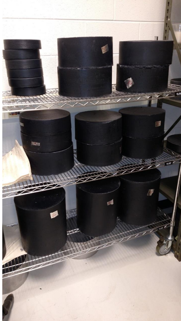
Figure 12 Small Solid fuel torch castings(upper left), ambient cooled grains(middle left) and some larger oven cooled grains(the rest).
