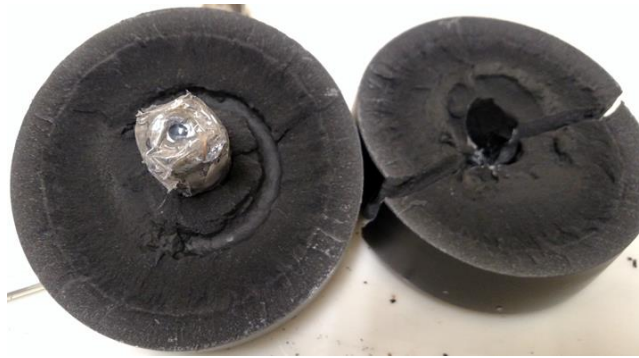
Figure 3 Early grain casting showing a mandrel design and grain cracking and voids.
