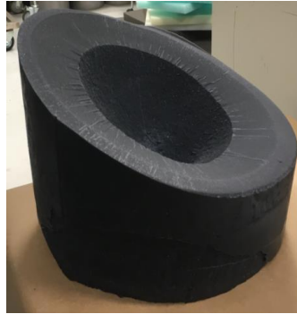
Figure 8 Monolithic grain after fracture, dome void. Upside down from cooling position.
