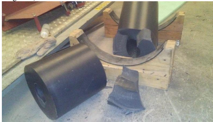
Figure 9 Fractured Monolithic Grain After Thermal Shock.
