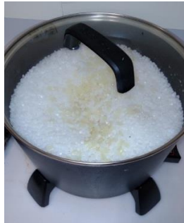
Figure 1 Early Melting attempts in a small, commercially available, deep fryer.
