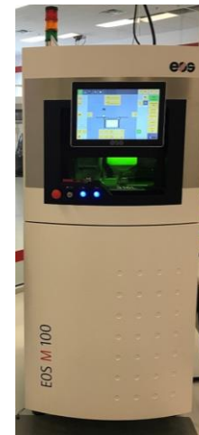
EOS M100 \varnothing 100x95 mm Power: 200 W Laser Diameter: 40 \mu m Material: Ti64, 316L, CoCr, W, Haynes 230. In-development: Monel K500, Haynes 282, Ta, W-25Re, Mo, Mo-41Re, Mo-47.5Re, C103, etc.
