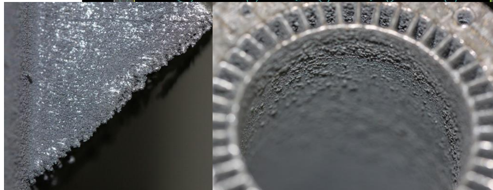
As-built surfaces of AlSi10Mg on Concept Laser X-Line.
