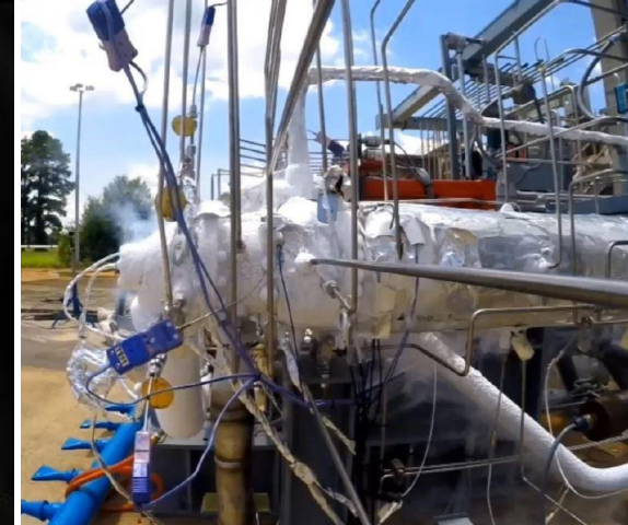
AMDE Fuel Turbopump Test. Courtesy Marty Calvert.
