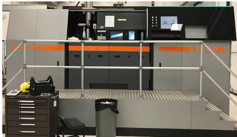
Concept Laser X-Line 1000R 630x400x500 mm Power 1000 W Laser Diameter : 70 \mu m Material: IN718
