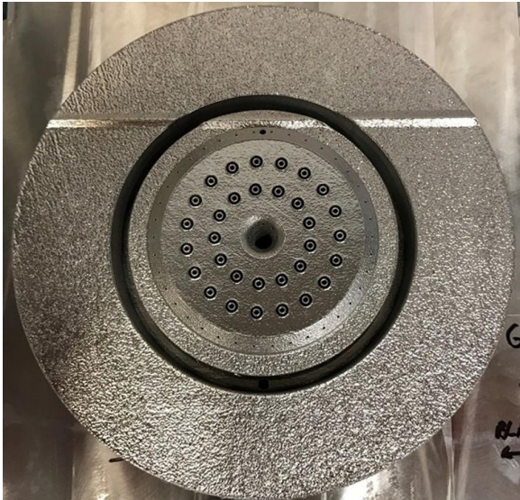
MET1 Injector V1 on EOS M290. Build time - $5.5k (55 hrs), Powder - $ 0.32k (5.82 kg), Saw - $0.2k, Plate resurface - $0.2k, Unsuccessful total - $6.22k. Successful total $6.22k. Total Cost $12.44k. 15 minute long simulation.
