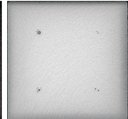
Known flaws in AISi10Mg block. Left: Regular CT. Right: Micro-CT
