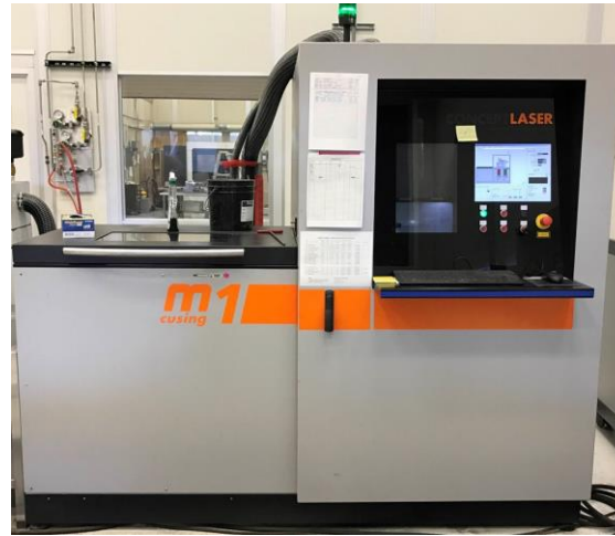
Concept Laser M1 250x250x250 mm Power: 400 W Laser Diameter: 70 \mu m Material: IN718, IN625, Monel K500.
