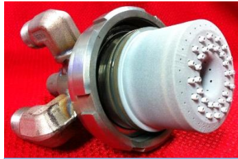
1.2K LOX/Hydrogen Injector First Tested in June 2013. >7200 seconds hotfire
