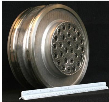
20K LPS Subscale Injector. Tested August 2013
