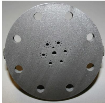
100lb LOX/Propane Nanolaunch Injector. Built 2012. Tested 2013.
