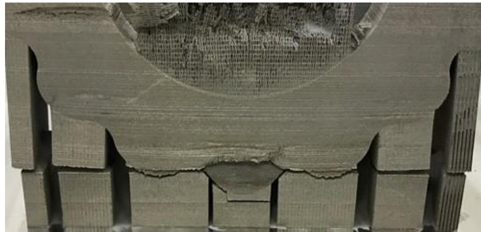
Residual stress induced failure.
