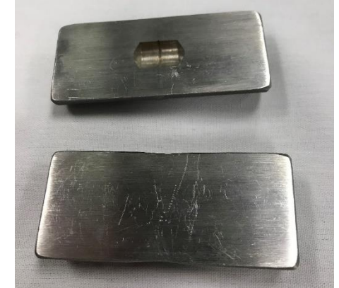
large machined cavity in a 1" diameter In625 bar that they were able to close with HIP; Courtesy Mark Battison (Quintus)
