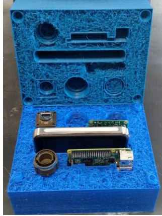
Figure 7. CRISSP 3D-printed foam developed by Tethers Unlimited. Image courtesy of Tethers Unlimited.
