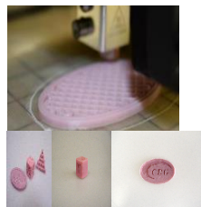
Figure 6. FDM prints using reclaimed anti-static bagging film with reversible cross-linking additive. Image from Cornerstone Research Group. Work conducted under an SBIR on development of recyclable packaging and common use materials for ISS.
