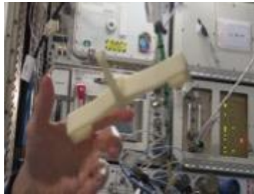
Figure 2. SPHERES Tow Hitch printed on ISS with AMF. SPHERES consists of 3 free-flying satellites on-board ISS. Tow hitch joins two of the SPHERES satellites together during flight. Printed 2/21/17.
