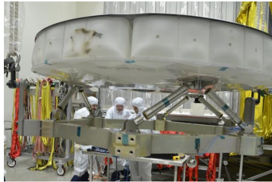
Figure 1-b. Test Article Suspended by Bungee
