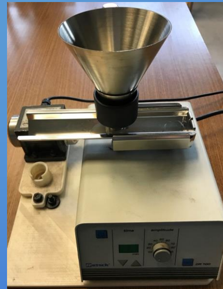
Vibratory Powder Fill Station
