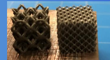
GRCop84 Met Cubes. (L) a = 5 mm, (R) = 2 mm.
