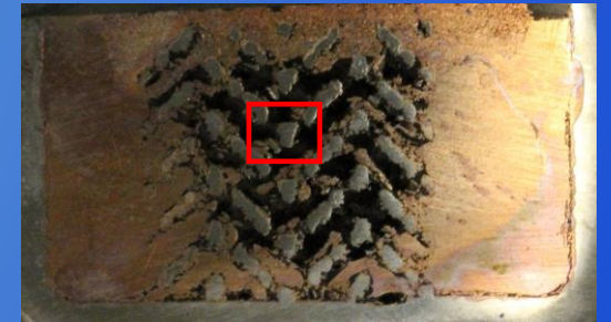
Rhombic Dodecahedron - 20%RD - 2 mm
