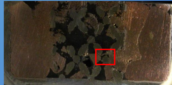
Rhombic Dodecahedron - 20%RD - 5 mm
