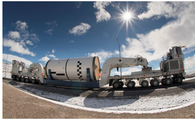
Figure 13. Northrop Grumman has nearly completed the five-segment solid rocket boosters for EM-1; motor segments will be shipped to Kennedy Space Center, where they will be stacked to assemble the final boosters.
