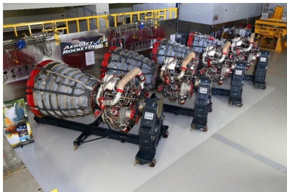
Figure 11. All four EM-1 RS-25 engines have been tested and verified; they are ready for integration into the core stage and flight.
