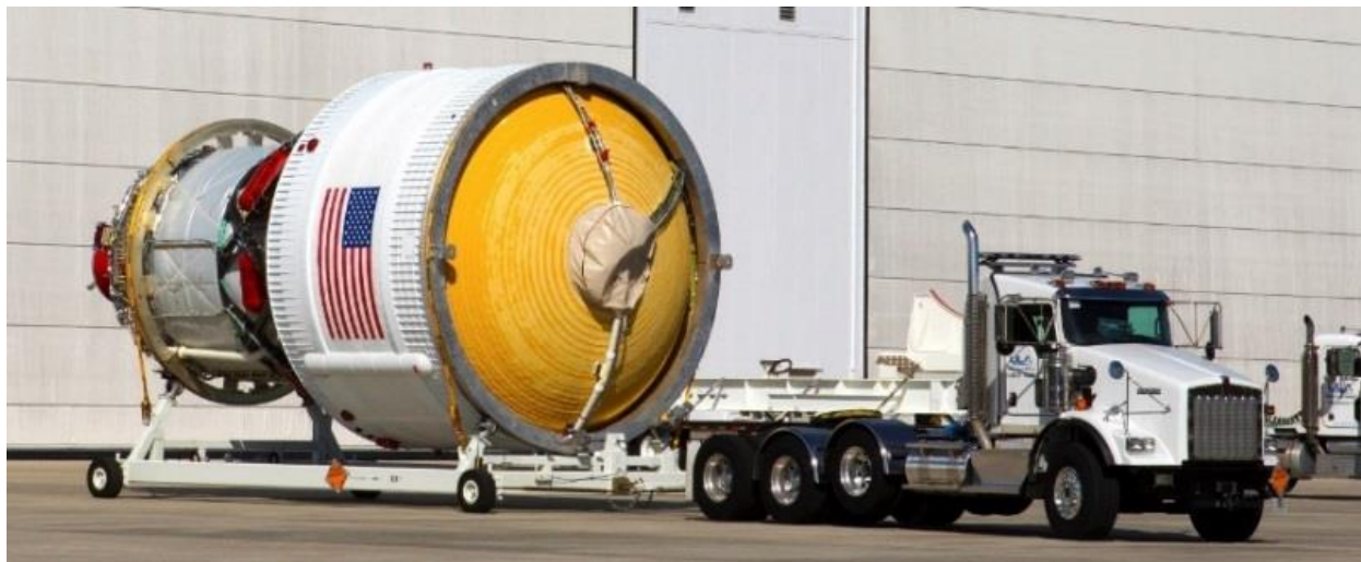
Figure 9. The ICPS, which will provide in-space propulsion for the first integrated flight of SLS and Orion, is complete.
