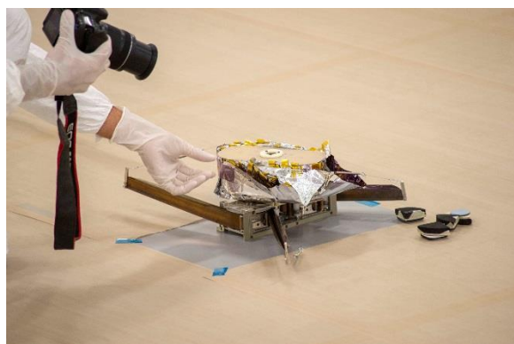
Figure 6. One of 13 6U-class secondary payloads manifested for EM-1, the NEA Scout spacecraft utilizes a solar sail the size of school bus on each side when unfurled.
