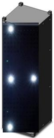
Target Spacecraft (3U CubeSat)
