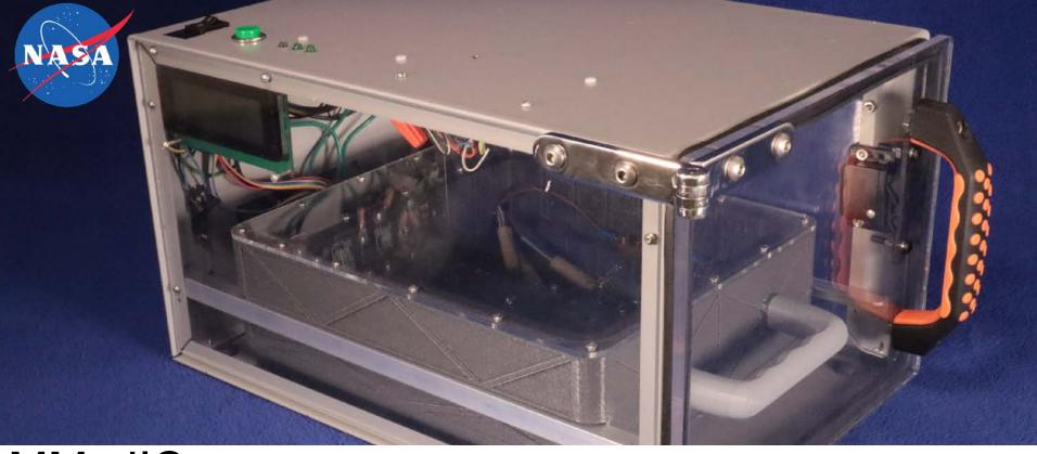
MMaJIC (Microgravity Materials Joining Investigation Chamber)
