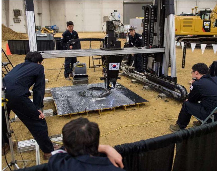
Figure 7. Gantry-style 3D printing system developed by Moon-X for the phase II, level 3 head to head competition.
