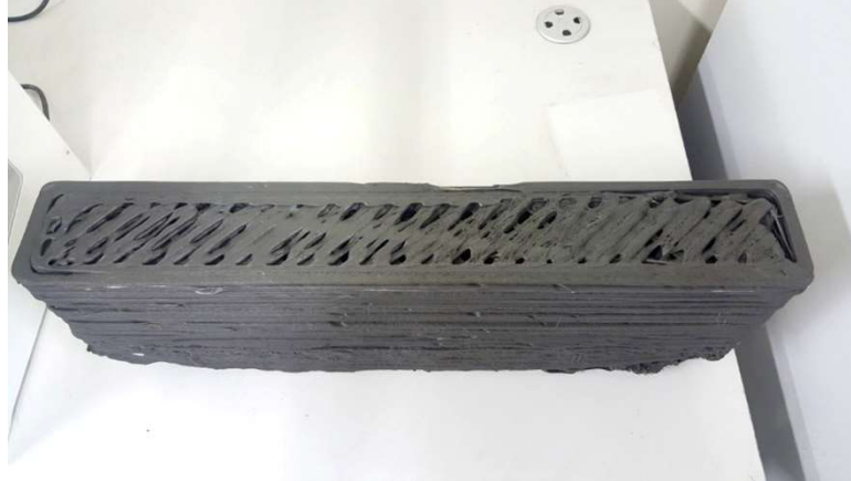
Figure 4. Beam specimen from Moon-X (South Korean team) submitted as part of phase II, level 2 structural member competition.
