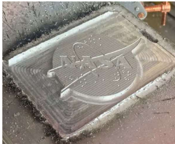
• Metal part produced with Vulcan manufacturing system. Image courtesy of MIS, Inc.
