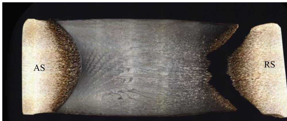
Figure 16. Fracture location in specimen no. 625-P07-RT06.
