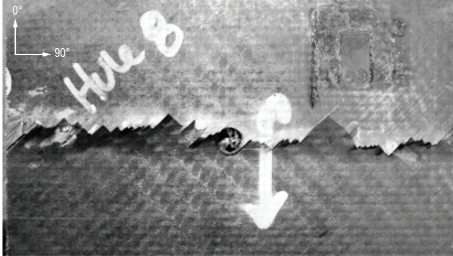
Figure 6. Photograph of failure zone of an open-hole compression specimen.
