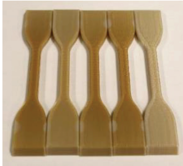
Figure 10. Two EM40 Ultem samples exposed to 500 ESH, two EM40 Ultem samples exposed to 1,000 ESH, and control sample.
