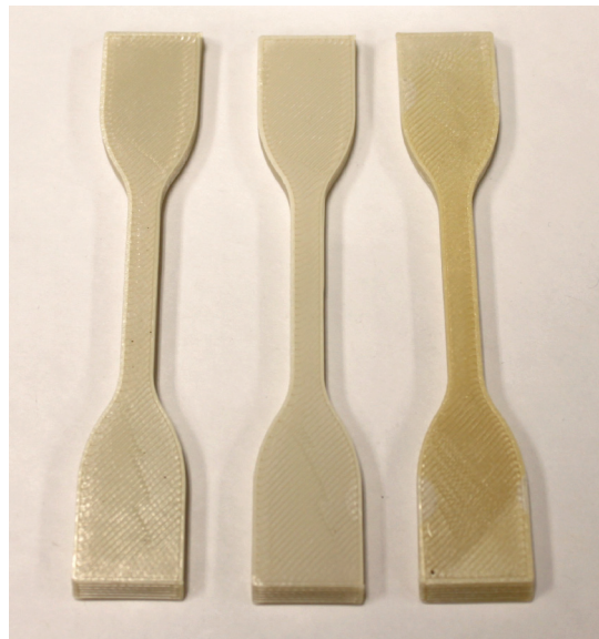
Figure 9. Left to right: MiS Ultem 9085 control sample, AO-exposed sample, UV-exposed sample.
