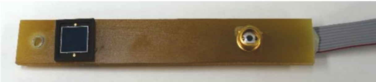
Figure 4. Left to right: Opto Diode UVG100 and UVG5S mounted on fiberglass, post-UV exposure.
