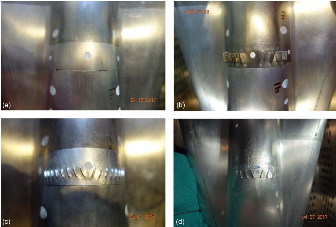
Figure 5.—Vortex generator configurations (see Table I for dimensions). (a) No VG. (b) C607 Baseline. (c) C607 Alternate. (d) C608 Baseline.
