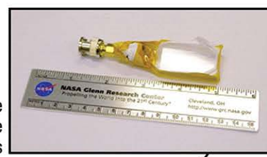
GaP diode for solid-state coincidence/anticoincidence detectors
