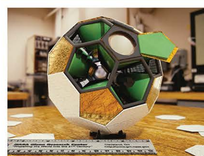
Space radiation detector with spherical geometry Technology covered by U.S. Patents 7,872,750 (January 18, 2011) and 8,159,669 (April 17, 2012)
