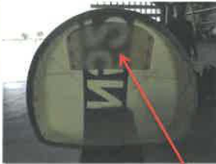
S-band wave-matching layer installed on fairing. This enabled S-band antenna mounting without any modifications to the already qualified fairing.
